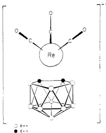
Figure 8. The structure of the  $\pi$ -(3)-1,2-dicarbollylrhenium tricarbonylate ion in schematic form.
