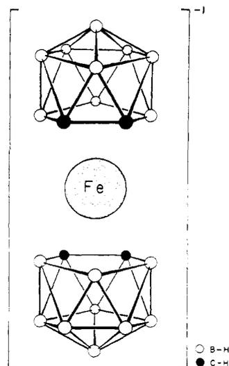
Figure 3. Proposed structure of the bis- $\pi$ -(3)-1,2-dicarbollyliron(III) ion in schematic form.
