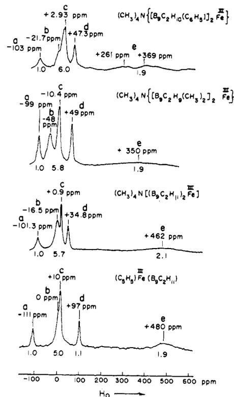
Figure 4. Boron-11 nmr spectra (19.3 Mc/sec) of iron(III) dicarbollyl derivatives. Chemical shifts were measured relative to  $BF_3 \cdot O(C_2H_5)_2 = 0$ .
